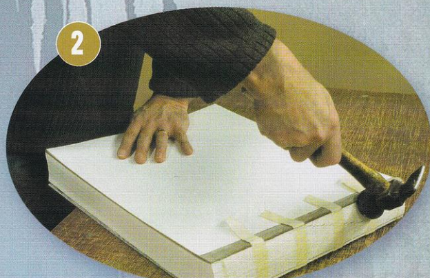
With fanatical care and precision, the binder manually "rounds" the spine of the sewn book block.
